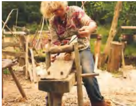
Drawkniving on the shavehorse to get it as near round as possible, so it is ready to turn
